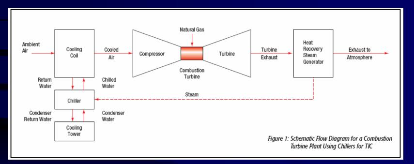
Figure Correction: There should be a stream for steam leaving the HRSG for use in steam turbine or other heating applications
