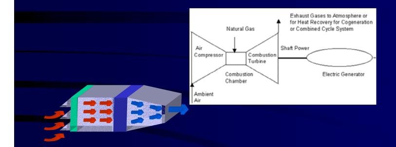
Cooling the inlet air to the compressor that supplies the high-pressure compressed air to the combustor of a combustion turbine
