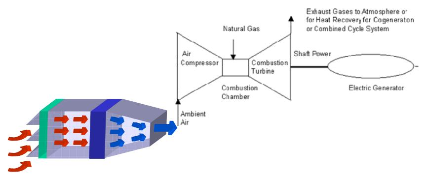
• Cooling the inlet air before or during compression in the compressor that supplies high-pressure compressed air to the combustor of a combustion turbine
