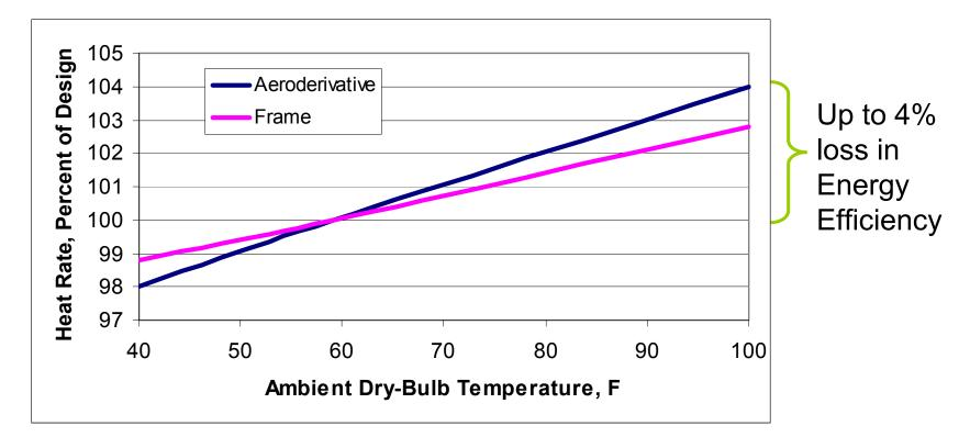
Note: Heat rate is directly proportional to fuel consumption per kWh and inversely proportional to energy efficiency
