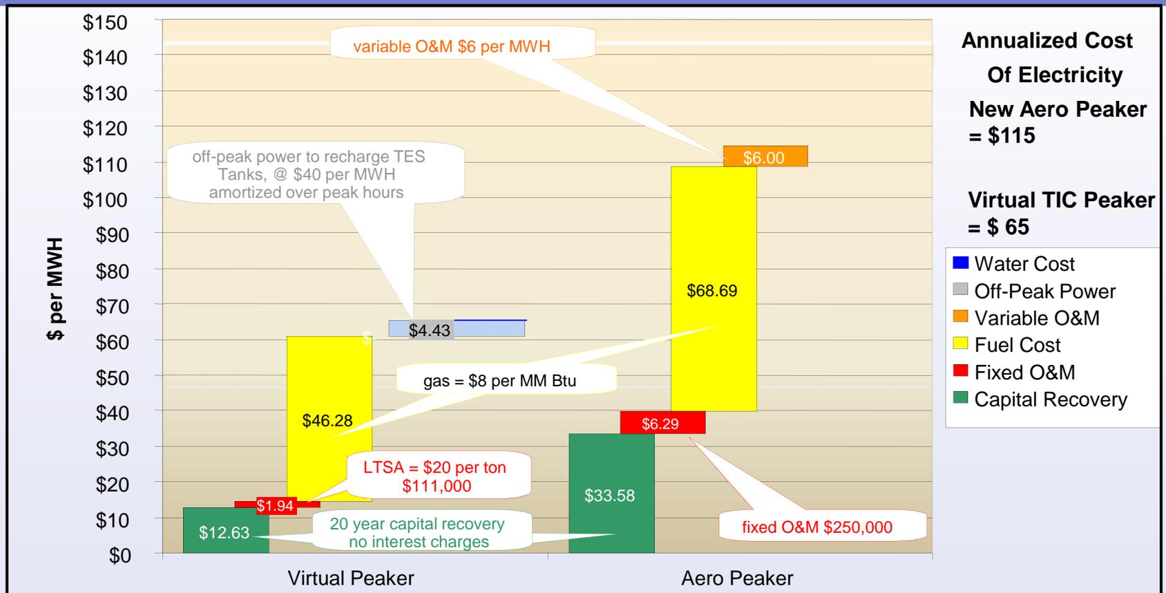
Basis: LM6000PC-Sprint with hot SCR & TIC vs. incremental MWH from combined cycle 207FA with TIC added. (Source: TAS)
