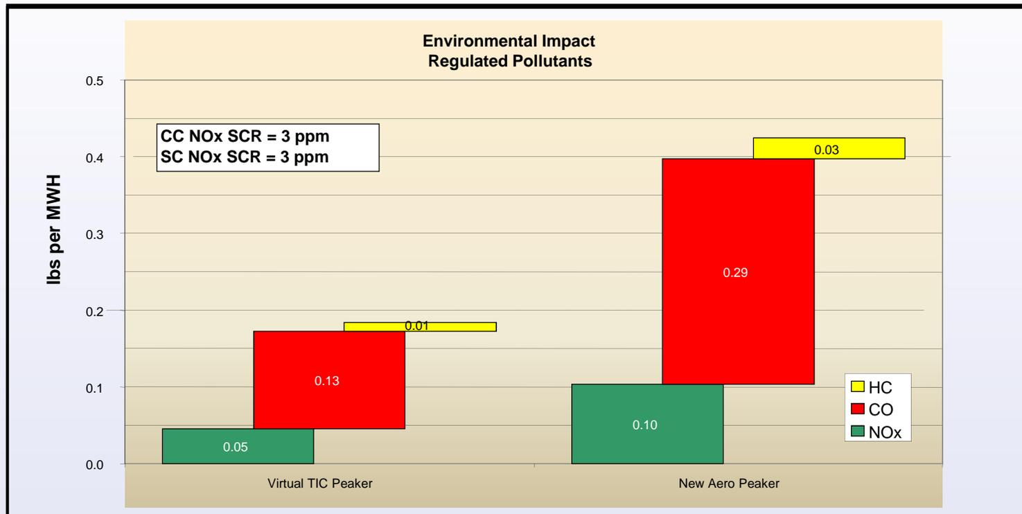
**TIC Reduces Total Emissions (lbs/MWh) by Over 50%**
