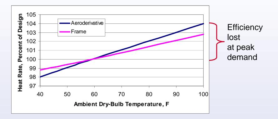
Note: Heat rate is proportional to fuel consumption per kWh
