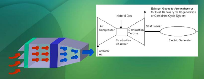
• Cooling the inlet air that enters the compressor section of the CT system
