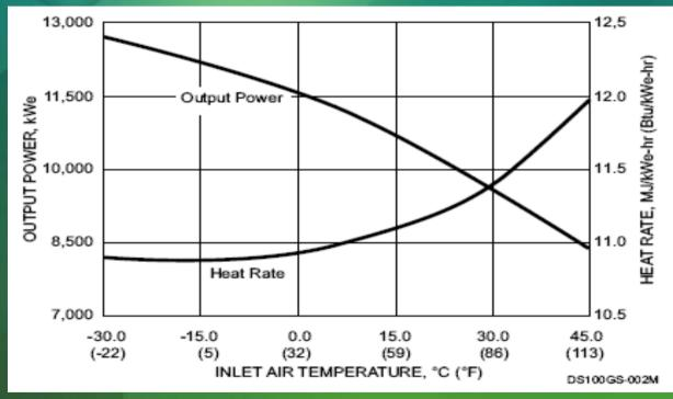
Efficiency loss of over 8 % from HR of ~ 11,100 to ~12,000 Btu/kWh
