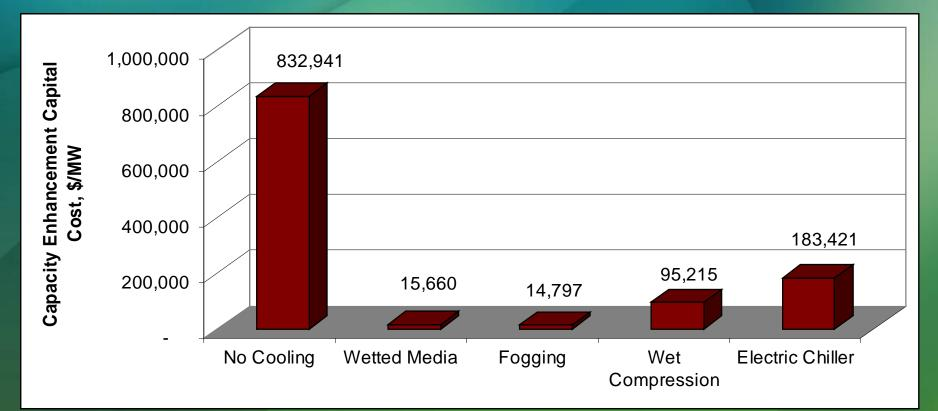
317 MW Cogeneration System Snapshot at 95°F DB and 80°F WB
