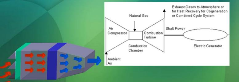
Cooling the inlet air before it enters the compressor or during its compression
